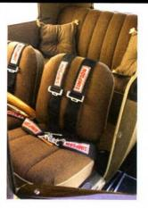
> Factory Model A seats may not provide a great deal of confidence during aggressive driving, but that's what the Simpson race harness is for. The belts are mounted discreetly and can be tucked out of sight. The misfire switch is located on the front of the shifter for easy access.
