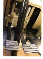
> The Tilton Engineering pedal assembly simplified the packaging for the new hydraulic brakes and clutch. The misfire circuitry that causes the engine to drop every third spark and sound remarkably like an original flathead-four is also hidden behind the dash with a removable panel for access.
