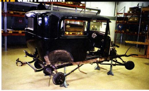
> The '29 was a solid base for a project, but 64 years in South America necessitated copious amounts of bodywork for rust and dent repair.
