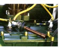
> The coup de grâce on the engine's masquerade is the original banger spark plugs mounted on the Cosworth valve cover with old-style cloth-covered wires. The ignition current passes right through and down to the Cossie's real plugs, which are deep in the cylinder head.
