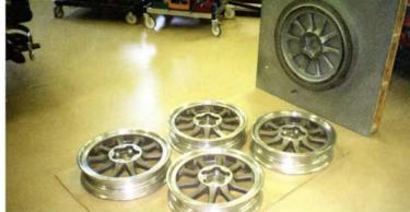
> Above and below: Wire or steel wheels would have been easier, but Kari wanted the absolute stealthiness of a wooden wheel. Of course wooden wheels will not hold up to this combination, so MAT built its own mold to cast the wheels in aluminum, then painted them to look like wood.
